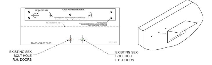
ALIGN EXISTING SEX BOLT HOLE ON THE DOOR, WITH IT'S CORRESPONDING HOLE LOCATION ON THE TEMPLATE (L.H. or R.H.). MARK AND DRILL HOLES FOR THE NEW SDC LOCK.
