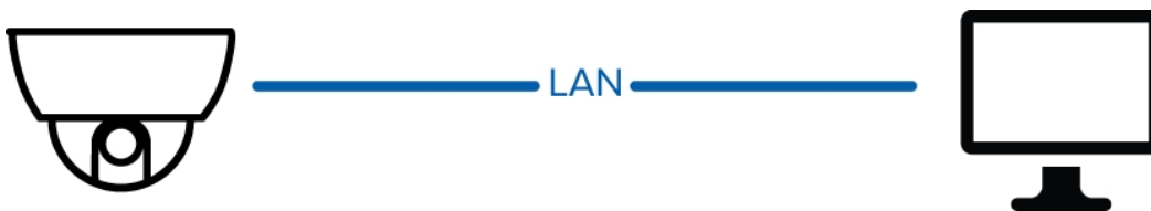
Figure 1: Single camera site. One H4 ES camera that can be accessed by the ACC Client on the local network.
