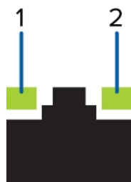
Figure 3: (1) Link LED. (2) Connection activity LED.
