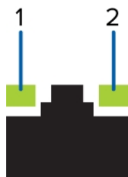
Figure 3: (1) Link LED. (2) Connection activity LED.
