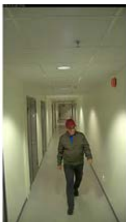
The above images are snapshots from AXIS Q1765-LE mounted indoors in a 30 m (98 ft) long hallway. The image to the left is the camera view in Corridor Format in wide view and day mode at 600 lux. The image in the middle, also in Corridor Format in wide view, is taken in night mode at 0 lux with IR illumination on and shows a person at a 2 m distance from camera. In the image to the right, the AXIS Q1765-LE is in Corridor Format and night mode at 0 lux with IR illumination on. The camera is in full tele view at 18x zoom and the person is at a 30 m.
