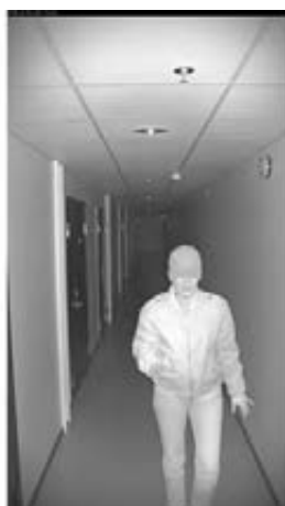
The above images are snapshots from AXIS Q1765-LE mounted indoors in a 30 m (98 ft) long hallway. The image to the left is the camera view in Corridor Format in wide view and day mode at 600 lux. The image in the middle, also in Corridor Format in wide view, is taken in night mode at 0 lux with IR illumination on and shows a person at a 2 m distance from camera. In the image to the right, the AXIS Q1765-LE is in Corridor Format and night mode at 0 lux with IR illumination on. The camera is in full tele view at 18x zoom and the person is at a 30 m.
