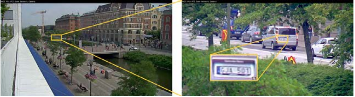
Images from AXIS P5414-E. Left: wide view. Right: 18x zoomed-in view where the license plate of a vehicle 200 m (660 ft.) away can be read.
