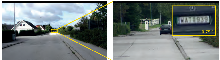
AXIS Q6035-E captures license plate of car 275 m (900 ft.) away. At left, a snapshot of the wide view in HDTV 1080p; at right, 20x optical zoom on a car with an inset of the license plate.
