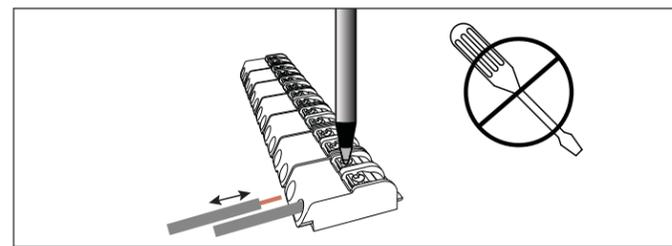
Figure 3.2: Inserting wire into the terminals
