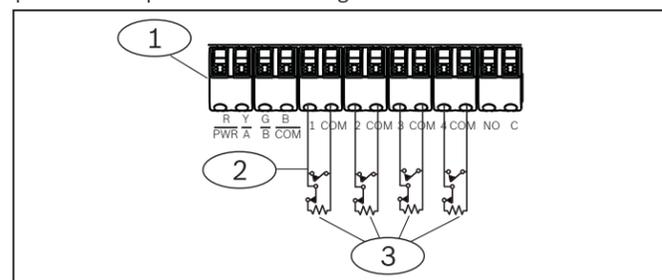
Figure 3.5: Installing sensor loop wiring
