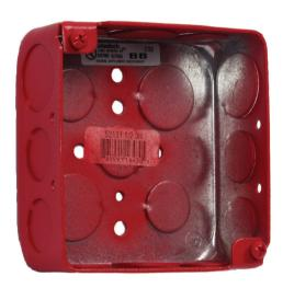
A painted steel back box with knockouts for interior surface mounting, concealed conduit mounting, or semi-flush applications. Measures 10.2 cm (4 in.) square by 3.8 cm (1.5 in.) deep.
