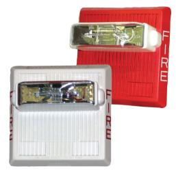
The Wheelock MT Mult-candela Electronic Appliances are audible and visual alarm-indicating devices engineered to comply with temporal pattern specifications without requiring an additional code mechanism. They have a selection of eight tone patterns, two sound output levels, and four light intensities (15 cd, 30 cd, 75 cd, or 110 cd). The temporal (Code 3) horn and tone patterns meet ANSI/ NFPA/ISO requirements for standard emergency evacuation signaling.
