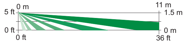
Side View Optional Barrier Coverage: 11 m x 3 m (35 ft x 10 ft)
