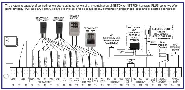
\*TSD = Transient Suppression Device (two supplied): Mount the TSD as close to the device to be protected as possible.
