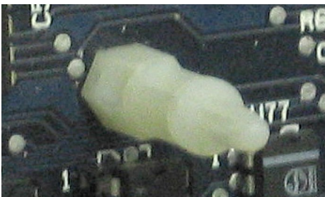
Fig. 7: Photo of one of the two white nylon snap-lock standoffs located at the upper-left of the PC motherboard.
