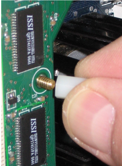
Fig. 10: Thread the thumb nut into the brass threads of the male-to-male standoff "finger tight".
