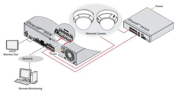
DirectIP™ NVR makes it easy to use cameras without extra network configurations.
