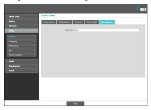
**Smart IR:** Set the brightness of the IR LED. The higher the value is set, the brighter it is.
