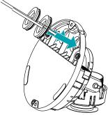
3 Use the screws, anchor provided with the camera to secure the bottom cover on a wall or a ceiling.
