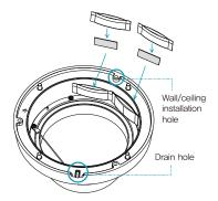
2 Fasten the screws for the dome cover clockwise using the Allen wrench provided with the camera.
