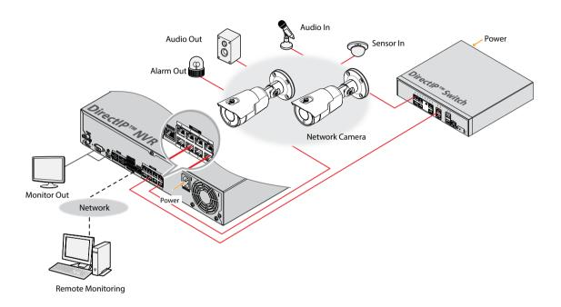
DirectIP<sup>™</sup> NVR makes it easy to use cameras without extra network configurations. Each camera can be controlled via the DirectIP<sup>™</sup> NVR setup menu, without any PC. For detailed camera settings, please see the camera setting pages of DirectIP<sup>™</sup> NVR manual.
