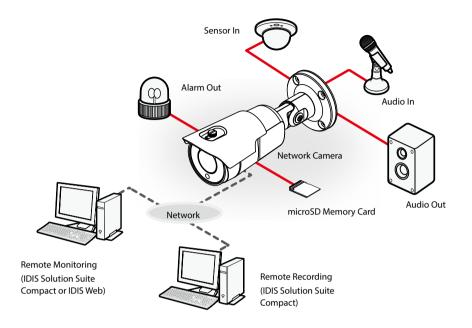
Control the camera over the network from software installed on a computer. Ideal for using the camera over the network from a remote location.
