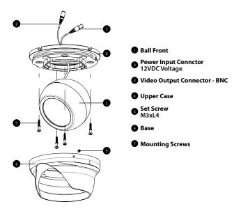
CAUTION: CHECK FOR POLARITY WHEN USING A DC12V POWER SUPPLY.
