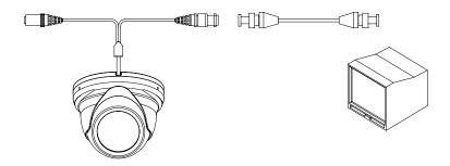
**CAUTION: CHECK FOR POLARITY WHEN USING A DC12V POWER SUPPLY.**
