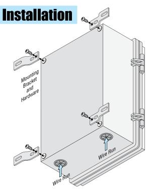
The plastic enclosure comes with mounting brackets and hardware to mount on enclosure. Mount enclosure on surface using appropriate hardware (not included). IT IS NOT RECOMMENDED DRILLING HOLES IN THE PLASTIC ENCLOSURE! If holes must be drilled, remove the circuit board before drilling and be sure that mounting bolts/screws do not touch the back of the circuit board. Holes must be sealed to prevent water intrusion.
