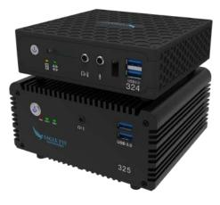
The Eagle Eye Cloud Managed Video Recorder (CMVR) stores video and acts as a gateway from your premises to the Eagle Eye Cloud Data Center where your video can also be stored and managed by the Eagle Eye Cloud VMS. It provides video storage, video buffering, a secure connection, bandwidth management, and monitoring of cameras.
