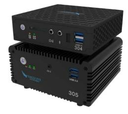
The Eagle Eye Bridge acts as a gateway from your premises to the Eagle Eye Cloud Data Center where your video is stored and managed by the Eagle Eye Cloud VMS. It provides video buffering, a secure connection, bandwidth management, and monitoring of cameras.
