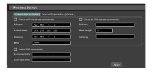
④ Go to Start → Settings → Camera → Add Camera. The NVR will automatically refresh the cameras searched. The IPC which supports the Onvif protocol may be added manually. If the IPC searched is not in the same local network as the NVR, you should select the device and click ■ to modify the IP address.
