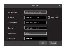
(5) Checkmark the device you want to add and then click "Add" button. The NVR will automatically refresh the cameras and return to "Edit Camera" interface. "Online" status means connecting the device successfully and you will see the live image. You may select the added device and click ▶ button to modify channel, IP address, etc.
