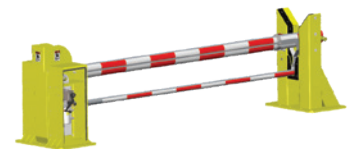
StrongArm M50 NP Manually operated ASTM F2656-07 M50-P2* 6 to 8 seconds Open/Close time 12 to 24 ft clear opening
