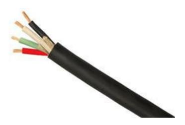
The C-XHHW-10-4 from Larson Electronics is 10/4 SOOW Industrial Service Cord that is available by the foot. This 10 AWG 4-Conductor Cable is 600V rated and can handle temperatures ranging from -40°C to +90°C for continuous operation, 130°C for emergency overload conditions and 250°C for short circuit conditions. This cord is for use Class I and II, Division 2 hazardous locations.
