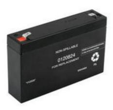
Dual Lite 0120824 Emergency Battery - 6 Volts - 7 Amp Hours - 3.4-Amps New, valve regulated, sealed lead acid (SLA) battery 6V, 7-7.2Ah capacity, F2 Faston terminals Supplies 3.4A at 6V for 90 minutes to an end voltage of 5.25V, per UL 924, Emergency Lighting and Power Equipment Meets pressure release requirements per UL 1989, Standby Batteries
