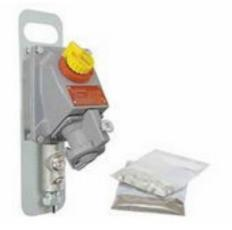
The Larson Electronics EPCO-3P4W-30A-ICB Portable Explosion Proof Connector Outlet provides a safe and secure power connection for portable or stationary electrical devices and equipment in hazardous locations. The 30-amp unit features a built-in circuit breaker and is constructed of copper-free aluminum. A backplate with carrying handle allows for easy transport within the jobsite.
