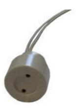
These sockets are specially made to fit the T8 Bulb/Prongs, as well as our own Larson Electronics LED tube lamps. The sockets allow the current to run to the tubes in order to produce light. These units fit the T8 fluorescent and the LEDT-15W, 2 foot bulbs. What makes these unique is that they are non-shunted, so they can be wired up for separate hot and neutral pins.
