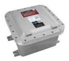
EPL-AEB-24.36.10-4X2S-1X0.75S Explosion Proof Enclosure Internal Dimensions: 24" L x 36" W x 10" H Weight: 100 lbs Mounting: Surface Mount Hubs: (4) 2" NPT, (1) 3/4" NPT (South Side of Enclosure) Features/Ratings Class I Division 1 Explosion Proof Class II Division 1 Explosion Proof
