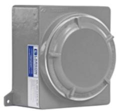
EPL-AEC-5.375-1X0.75S-1X2B Explosion Proof Device Box Instrument Enclosure - Class I, II, III Div 1 & 2 Listing: NRTL Listed for United States and Canada; ATEX/IECEx Rated Device Type: Explosion Proof Instrument Enclosure External Dimensions: 9.13" x 9.63" x 7.18" Internal Dimensions: 7.06" x 8.31" x 4.13" Lens Opening: 5.38" Internal Volume: 305 cu. in. Weight: 60 lbs.
