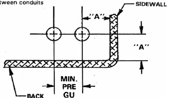
**Chart 2: Required wall thickness for five (5) full threads engagement per U.L. 886 Standards.**
