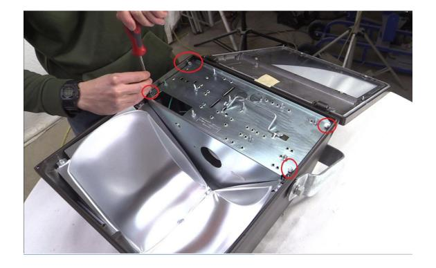
**3.** Then grab the handle and lift the inside of the light out. The ballast will be attached to this removable faceplate. The faceplate will still be secured to the housing by a ground screw and zip-tie both circled in red in the pictures below.
