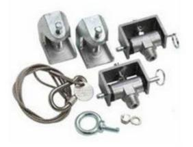
The EPL-xx-2L-SP0195 is a replacement drop mount kit for Larson Electronics EPL-48-2L and EPL-24-2L series explosion proof lights. This kit is used to lower a fixture on one side for lamp servicing and includes two pin release mounts for the fixture, two safety cables, and two safety cable mounts. Two kits are required for 4 lamp fixtures.
