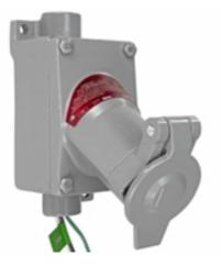
EPO-20A Explosion Proof Outlet - Delayed Action/Straight Blade Listing: NRTL Listed for United States and Canada Dimensions: 5 3/4" x 3" Weight: -Voltage: 125V or 250V Amps: 20A Poles: 2P Wires: 3W Protection: Spring-loaded Cover Materials: Copper Free Aluminum Finish: Electrostatically Applied Baked Powder Epoxy/polyester Mount: (4) 1/4" Mounting Holes
