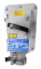
EPO-60A-3W4P-CB.LS Explosion Proof Receptacle Unit Type: Explosion Proof Receptacle w/ Interlocked Circuit Breaker Dimensions: 16.83" x 9.06" x 13.95" Weight: -Voltage Rating: 600V AC/250V DC Amp Rating: 60A Configuration: 3-wire, 4-pole
