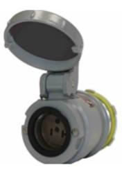
EPO-PM-20A-FC Explosion Proof Outlet - Delayed Action/Straight Blade Listing: NRTL Listed for United States and Canada Dimensions: 5" x 3 11/16" Weight: -Voltage: 125V or 250V Amps: 20A Poles: 2P Wires: 3W Protection: Flip Cover Materials: Copper Free Aluminum Finish: Electrostatically Applied Baked Powder Epoxy/polyester Mount: Panel Configuration: -
