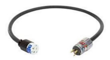
EPP-20A Explosion Proof Plug Amp Rating: 20 Dimensions: 2.78"-L 1.75"-W Configuration: 3 Pole 2 Wire Suitable Cable Diameter: .538" to .639" Wiring: 3ft Pigtail - 12/3 SOOW Cord Comparability: EPO-20A Receptacle- Crouse Hind™ ENR Receptacles Cross Interchangeability: Crouse Hind™ENP5201 and Hubble Killark UGP-20231-UGP-20232 ACCEPTOR® plugs
