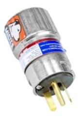
EPP-15A Explosion Proof PLug Amp Rating:15 Dimensions: 2.78"-L 1.75"-W Configuration: 3 Pole 2 Wire Suitable Cable Diameter: .538" to .639" Voltage Rating: 125V 1HP or 250V 2HP Compatability: EPO-15A Receptacle- Crouse Hind™ ENR Receptacles Cross Interchangeability: Crouse Hind™ENP5201 and Hubble Killark UGP-20231-UGP-20232 ACCEPTOR® plugs
