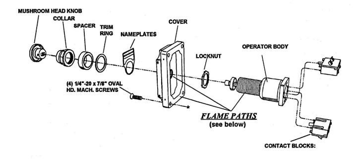
A FLAME PATH IS MACHINED ON BOX & COVER SUCH THAT A 0.0015" FEELER GAUGE WILL NOT ENTER THE JOINT MORE THAN 1/8" WHEN FULLY ASSEMBLED AND BOLTED. CARE MUST BE TAKEN THAT MACHINED SURFACES AND THREADED AREAS ARE NOT DAMAGED.
