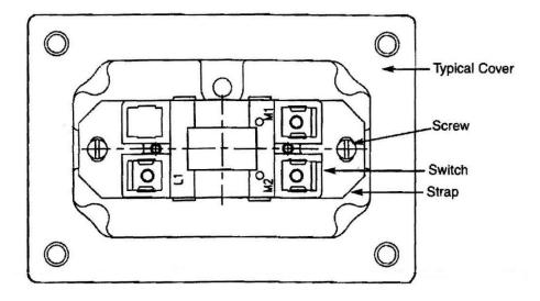
**CAUTION:** Use 12 AWG copper conductors only. Insert the bare wire conductor(s) under the terminal clamp and securely tighten the screw(s). Note: Do not exceed 35 in-lbs. of torque. Wire according to diagram on switch.
