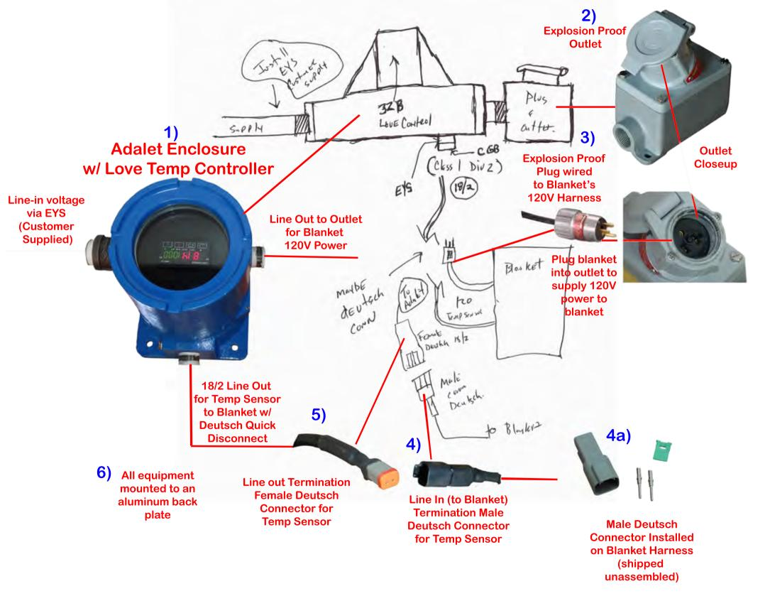
1) Adalet enclosure w/ customer supplied Love temperature controler 2) Explosion Proof Outlet to supply **120V power to blanket** 3) Explosion Proof Plug attached to installed wiring harness on blanket Plug is shipped uninstalled and customer must install plug to blanket harness 4) Male 2-pin Deutsch connector installed on wiring harness for temperature sensor cable on blanket 4a) Male Deutsch connector shipped
