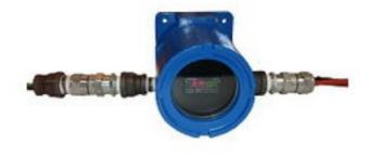
Explosion proof enclosure with Love temperature control system. The end user provides control voltage through the second NPT. The power flows to the Love controller and then to the appliance via the 20 amp explosion proof outlet. Temperature sensing cables supplied by end user are passed through another NPT and are terminated at the Love controller.
