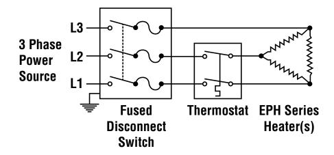
Three Phase AC heater circuit where line voltage and current do not exceed thermostat rating. Circuit does not have a "positive" off.
