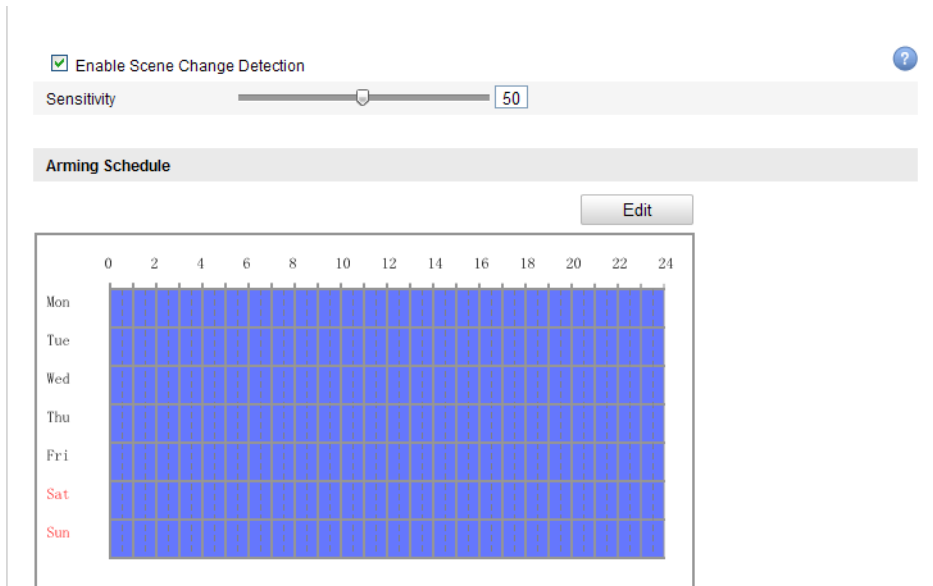
Figure 6-60 Configuring Scene Change Detection
