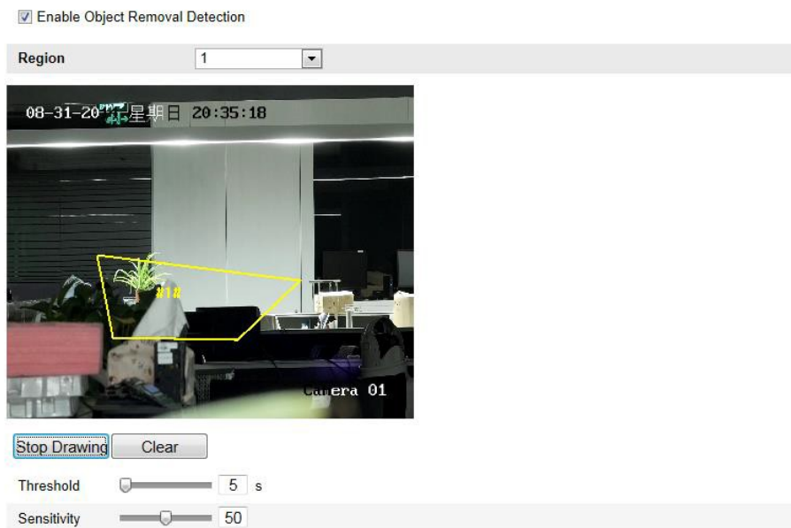
Figure 6-67 Configuring Object Removal Detection
