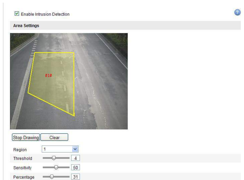
Figure 6-63 Configuring Intrusion Area
