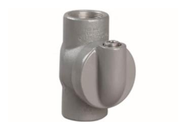
3" Explosion proof seal off is used to make a junction between an explosion proof lights and rigid pipe. Typically, users will make their connections, keep the conductors separate and pour chico into the seal off.
