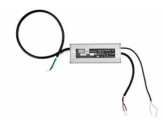
HALS-EMG-48-2L-LED-SP0109 LED Driver Type: Replacement LED Driver Dimensions: 1.18"-H × 9.47"-L × 1.68"-W Maximum Output (Watts): 96W Input Voltage Range: 90-305 V AC Output Voltage Range: 12-24 V DC Typical Efficiency: 87% Power Factor: 0.99 @ 120 V AC, 0.99 @ 220 V AC
