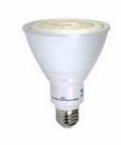
LED-PAR30-15-E26-120V 20 Watt LED Bulb Lamp Type: LED Watts: 20 Lumens: 750 Dimensions: 4.75" in diameter Beam Config: 40° Voltage: 120 VAC Color: 3000K CRI: >84 (White)
