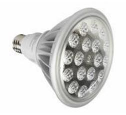
LED30W-PAR38 25 Watt LED Bulb Lamp Type: LED Watts: 25 Lumens: 2500 Dimensions: 4.75" in diameter Voltage: 11-25V AC/DC Color: White (Red, Green, Blue, Amber, and Infrared also avaliable.) CRI: >84 (White) Operating Temp: -20C to 85C
