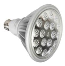
LED30W-PAR38-125VDC LED PAR38 Lamp Type: LED Watts: 25 Lumens: 2500 Dimensions: 4.79" (121.65mm) OD 4.74" (120.32mm) Total Height- 3.61" (91.64mm) Voltage: 125V DC Color: White (Red, Green, Blue, Amber, and Infrared also available. There may be longer lead times on specialty colors) CRI: >84 (White) Operating Temp: -20C to 85C Materials: Aluminum Housing - Polycarbonate Lens Dimmable: No
